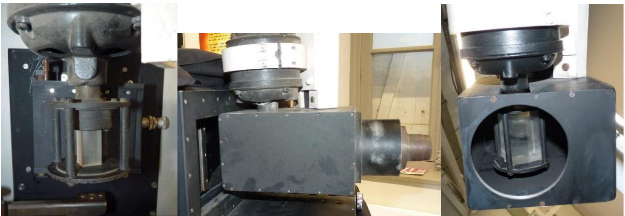
Figure 11 : the rotating prism in front of the entrance slit F of the spectrograph (left), the ocular (centre) and the rotating prism at the output slit F_2 (right). Courtesy OP.
